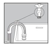
3. Place the discharging hose in a washbasin or sink with the aid of the bent piece delivered separately. The bent piece has to be entered into the tube's mouth in order to assure the support. Aforesaid piece allows the hose to be fixed to the wall by means of an opening on the upper part and that way the hose does not move and its falling is avoided.
